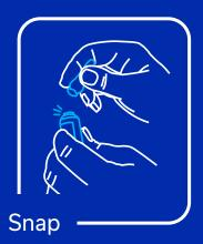
Open a new ampule before each test. These can be used straight out of the box and are specifically made to work with our Advanced Instruments osmometers.
