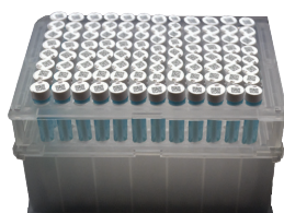
Raise E-Z 96 ® Spin-Out plate adaptor and centrifuge to separate lysis buffer (containing DNA) and swab. Swabs and plate adaptor may be discarded.
